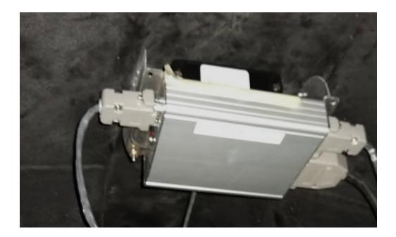
Engine-specific sensor inputs are being produced by two ECUs (ECU1 and ECU2 which are programmed similarly (but not identically) for redundancy). The ECUs come from the marine industry and are GM/Delphi/ACDelco **Marine Electronic Fuel Injection** (MEFI) which are used to control Volvo Penta, Indmar and other marine engines. In Talon A600 version 4 of the MEFI is used.
