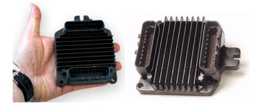
The ECUs provide Full Authority Digital Control (FADEC) over the engine, i.e. it controls the amount of fuel being injected (fuel mixture ratio), timing advance and other parameters based on the sensor inputs.
