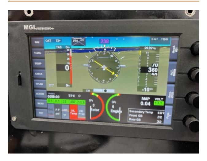
EFIS is able to provide these functions based on the inputs from various sensors, some of the sensors are built-in into the unit (for example Outside Air Temperature), and some are received signals.
